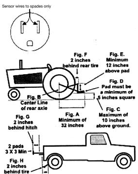
NOTE: The stabilizer bar system must be able to support the weight of the machine in the heaviest class pulled. Jacking up the pads, so machine is completely off the ground, will be a good test.
